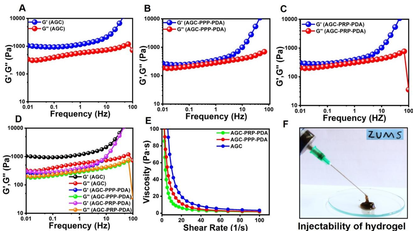
Fig. 4 Rheological performance of the hydrogels. (A) Frequency sweep test of (A) AGC, (B) AGC-PPP-PDA, and (C) AGC-PRP-PDA hydrogels. (D) Rheological performance of the hydrogels determined by employing an oscillation-frequency test. (E) Shear thinning assay of the hydrogels. (F) Injectability test of the AGC-PPP-PDA hydrogel using a 27-G needle.
