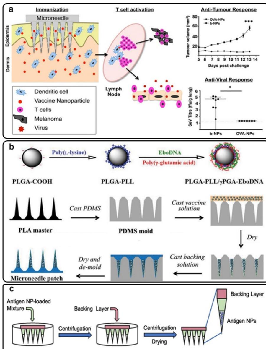
**Fig. 7** (a) Antitumor and anti-viral immune responses of skin dendritic cells targeted via PLGA MNs; reproduced from ref. 64 with permission from ACS, copyright 2013; (b) the preparation procedure for PLGA-PLL/γPGA-EboDNA dissolving MNs; reproduced from ref. 66 with permission from Wiley, copyright 2017; (c) influenza matrix 2 (M2) antigen nanoparticle-loaded PLGA MNs; reproduced from ref. 69 with permission from Elsevier, copyright 2022.
