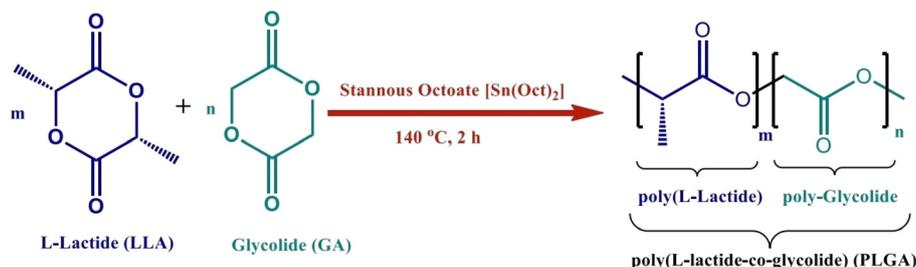
Fig. 2 Synthesis and structure of PLGA. Reproduced from ref. 34 with permission from MDPI, copyright 2021.
