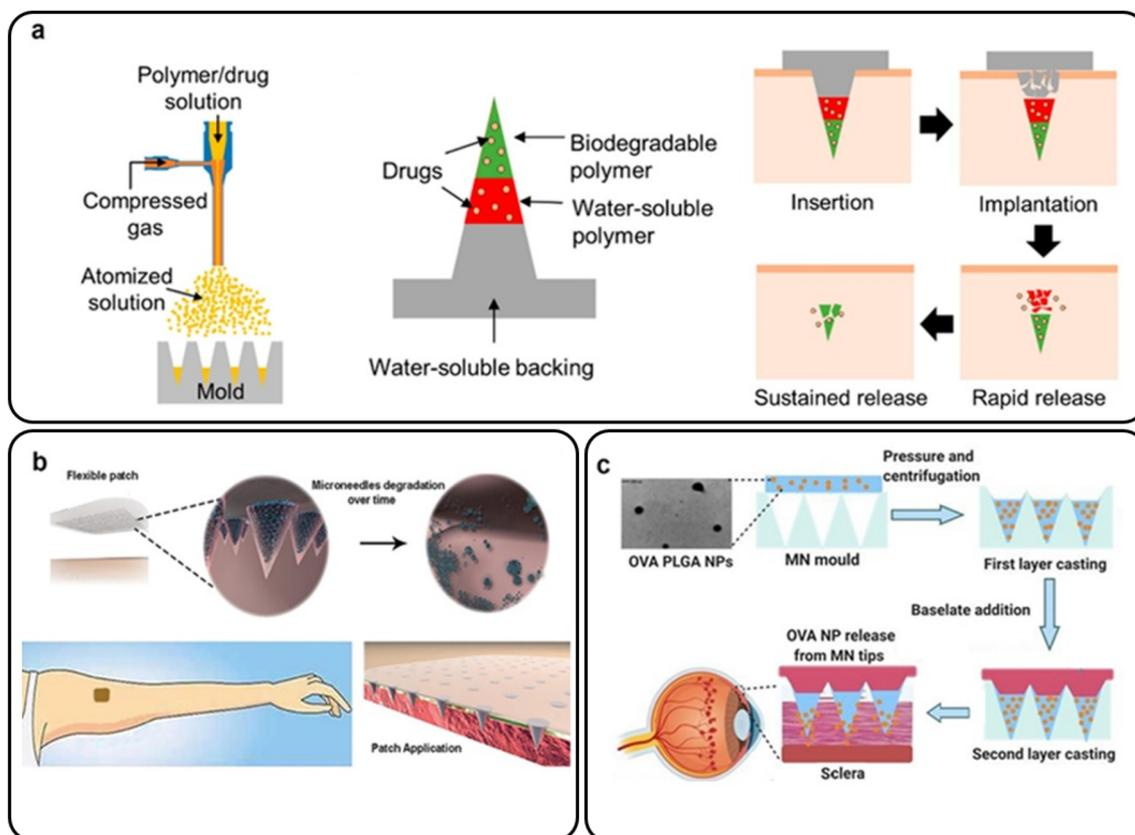
**Fig. 12** (a) Layered PLGA/PVP MNs for the transdermal delivery of BSA. Reproduced from ref. 113 with permission from MDPI, copyright 2019; (b) an array of MNs containing biodegradable PLGA microparticles for intradermal delivery of POXA1b laccase. Reproduced from ref. 114 with permission from Frontiers Media S.A., copyright 2019; (c) bilayer OVA-encapsulated PLGA nanoparticle-based MN arrays. Reproduced from ref. 118 with permission from Elsevier, copyright 2021.
