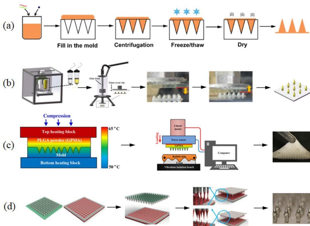
**Fig. 9** Method for the preparation of microneedles. (a) Molding. (Adapted with permission from ref. 91. Copyright © 2021, the American Chemical Society.) (b) 3D printing. (Adapted with permission from ref. 88. Copyright © 2020, Elsevier B.V. All rights reserved.) (c) Hot pressing. (Adapted with permission from ref. 92. Copyright © 2019, Elsevier B.V. All rights reserved.) (d) Extrusion stretching.<sup>93</sup> Copyright © 2015, IOP science.
