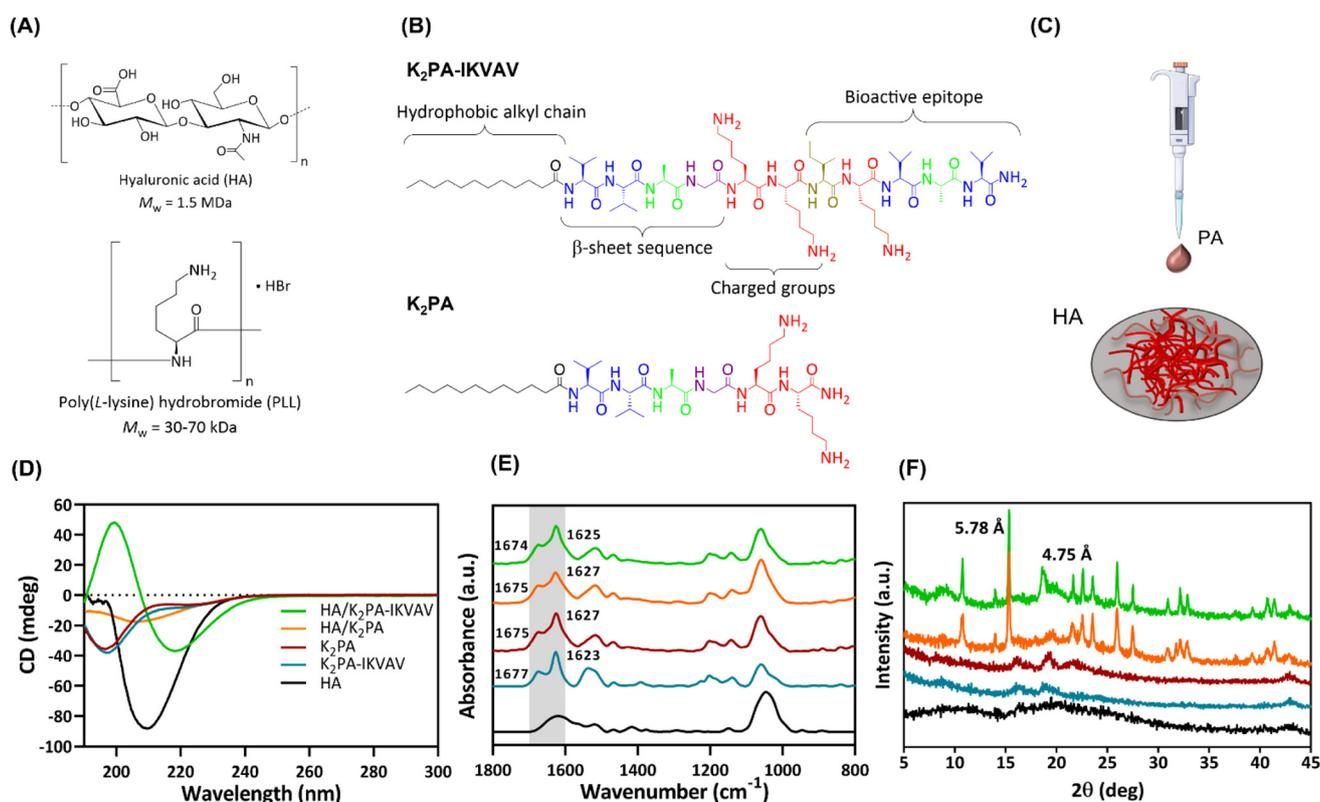
**Fig. 1** (A) Chemical structures of HA and PLL and (B) bioactive ( $K_2$ PA-IKVAV) and non-bioactive ( $K_2$ PA) PAs. (C) Schematic illustration of the preparation of either HA/ $K_2$ PA or HA/ $K_2$ PA-IKVAV supramolecular co-assemblies. Secondary structure analysis of the individual components and co-assembled systems using (D) CD, (E) ATR-FTIR, and (F) WAXS.
