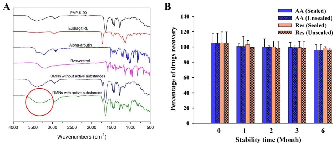
**Fig. 6** (A) FTIR spectra in the range of 4000–500 cm<sup>-1</sup> from PVP K-90 powder, Eudragit RL powder, AA powder, Res powder, unloaded DMNs, and AA/Res-loaded DMNs and (B) stability study of AA/Res-loaded DMN patches (F3) under sealed and unsealed conditions at 25 °C ± 2 °C and 60% ± 5% RH for 0, 1, 2, 3, and 6 months (mean ± SD, *n* = 3).
