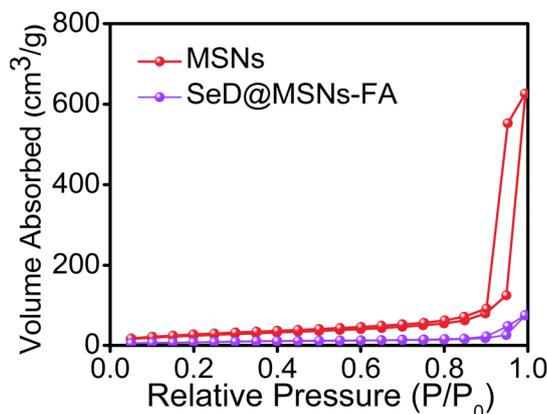
Fig. 1 (G) N<sub>2</sub> adsorption–desorption isotherm.
