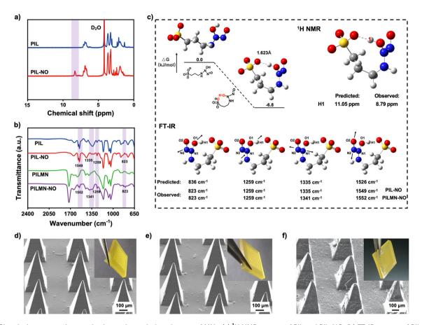
Fig. 1 Chemical structure characterization and morphology images of MNs. (a) <sup>1</sup>H NMR spectra of PIL and PIL-NO. (b) FT-IR spectra of PIL, PIL-NO, PILMN and PILMN-NO. (c) Energy gap between two different structures of [APS]-NONO. Prediction of the FT-IR vibration model and <sup>1</sup>H NMR spectra for [APS]-NONO. SEM images of the freshly prepared (d) PILMN, (e) PILMN-NO and (f) PILMN-NO after insertion into the isolated skin (insert: corresponding images).
