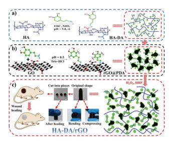
**Fig. 3** Diagrammatic sketch of HA-dopamine/rGO hydrogel preparation. (a) Preparation scheme of the HA-dopamine polymer and (b) rGO@PDA, (c) scheme of the HA-dopamine/rGO hydrogel and the original, bending, compressing, and self-healing representations and the application in wound healing. Scale bar: 5 mm. Reprinted with permission from the reference *Small*, 2019, **15**, 1900046. Copyright 2019 John Wiley and Sons.
