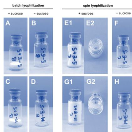
**Fig. 3** Cake appearance of freeze-dried eGFP mRNA-LNP formulations via conventional batch lyophilization S-Ac7-Dog formulation (A) with sucrose and (B) without sucrose, S-Ac7-DHDA formulation (C) with sucrose and (D) without sucrose; and via spin lyophilization S-Ac7-Dog (E1 and E2: top view) with sucrose and (F) without sucrose, S-Ac7-DHDA (G1 and G2: top view) with sucrose and (H) without sucrose.
