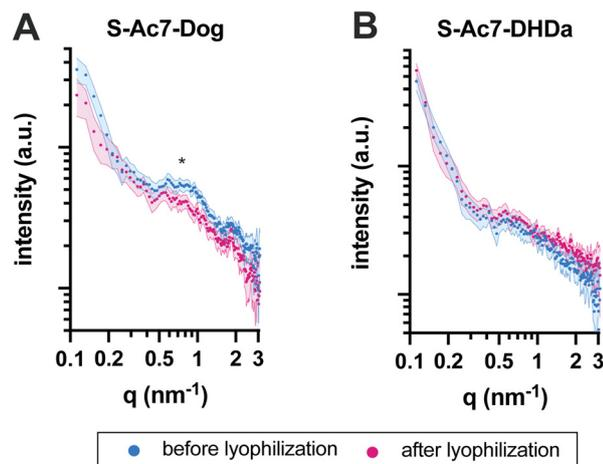
**Fig. 5** SAXS patterns for the mRNA-loaded (A) S-Ac7-Dog and (B) S-Ac7-DHDa LNPs before (blue) and after (pink) lyophilization. Correlation peak attributed to mRNA arrangement within the LNPs is marked with an asterisk.
