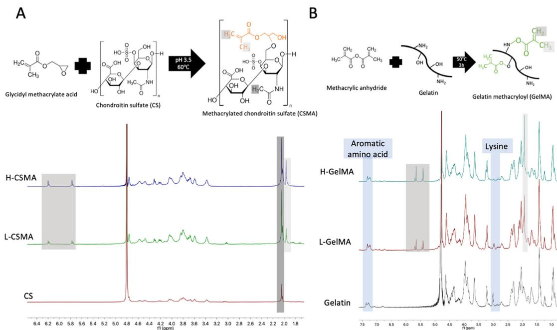
**Fig. 1** Synthesis and  $^1\text{H}$  NMR spectra of CSMA (A) and GelMA (B). The white and grey shadows marked the peak ascribed to the methyl group adjacent to the double bond and the double bond; the black shadow marked the methyl group on the original CS.
