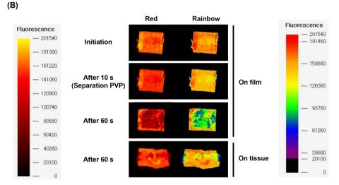
Fig. 8 Ex vivo study for EVL transfer onto tissue using UTM. (A) Customized UTM set-up to simulate drug transfer onto the tissue of porcine aortic arteries from a PVP/EVL-NO-Lipo/PVP-coated film. (B) Time-dependent fluorescence images of the film and tissue to confirm separation of the 3rd PVP layer and 2nd EVL-NO-Lipo layer (Red: Nile-red labeled liposome).
