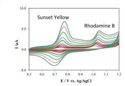
Applicability of a graphene oxide nanocomposite for fabrication of an electrochemical sensor for simultaneous detection of sunset yellow and rhodamine B in food samples
