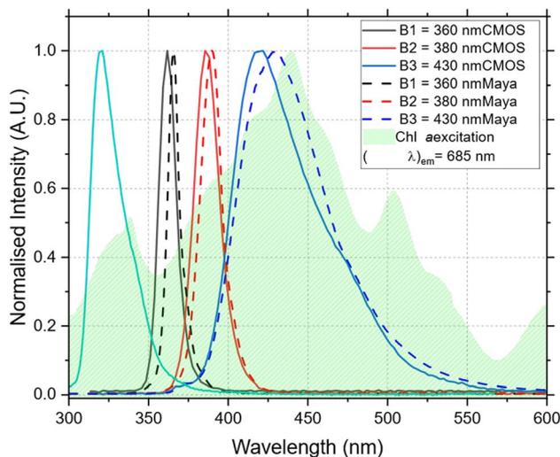
Fig. 2 Spectrum of each LED used in this study as recorded on the Hamamatsu mini-spectrometer and the Ocean Optics Maya 2000 PRO Series spectrometer. Overlaid is the *in vivo* excitation spectrum of cultured diatomic algae ( $\lambda_{em} = 685$  nm).
