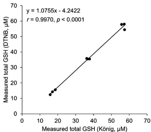
Fig. 5 Correlation between the present method and the DTNB method. Total GSH concentration in the same sample was quantified by the present method ( $x$ -axis) and the DTNB method ( $y$ -axis). Pearson's correlation analysis was performed.
