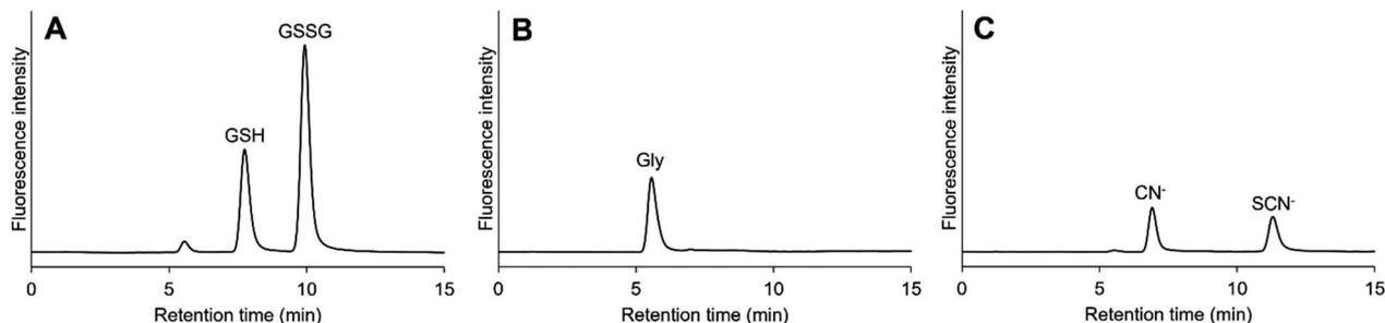
Fig. 2 Typical chromatograms of reduced and oxidized glutathiones (GSH and GSSG), glycine (Gly), and cyanide and thiocyanate ( $\text{CN}^-$  and  $\text{SCN}^-$ ). (A) 5  $\mu\text{M}$  GSH and 5  $\mu\text{M}$  GSSG, (B) 0.1  $\mu\text{M}$  Gly, (C) 0.1  $\mu\text{M}$   $\text{CN}^-$  and 0.1  $\mu\text{M}$   $\text{SCN}^-$ . Column: Scherzo SM-C18 (3  $\mu\text{m}$ , 150  $\times$  4.6 mm i.d.). Mobile phase: 75 mM acetate buffer (pH 5.0).
