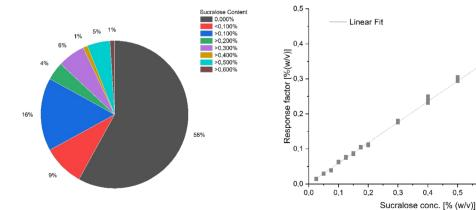
Fig. 1 Sucralose content of e-liquid samples derived from HPLC-MS/MS measurements (left) which were quantified using a linear fitted matrixmatched calibration (right).
