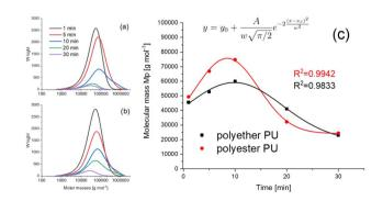
Fig. 5 Molar mass distribution curves of a polyester PU (a) and a polyether PU (b) and the course of the molar mass changes monitored by SEC over time (c) with  $y_0 = 18950$  (24220),  $x_c = 10$  (8), w = 19 (12) and  $A = 9.43 \times 10^6$  (7.86  $\times$  10<sup>6</sup>) for the polyether (polyester) PU.
