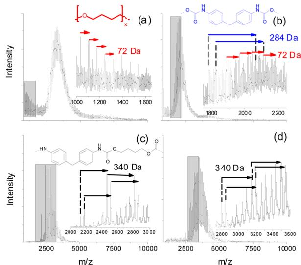
Fig. 4 MALDI TOF mass spectra of lower mass SEC fractions of purified (by precipitation in MeOH) polyether and polyester PUs after thermal treatment at 150 °C (7 d): (a and b) polyether PU, (c and d) polyester PU.
