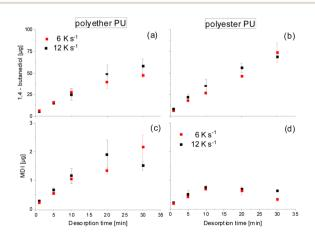
Fig. 3 Time-dependent thermal desorption at 250  $^{\circ}$ C of 1,4 butane-diol and MDI from polyether PU (a and c) and polyester PU (b and d) at heating rates of 6 (red) and 12 K s<sup>-1</sup> (black).
