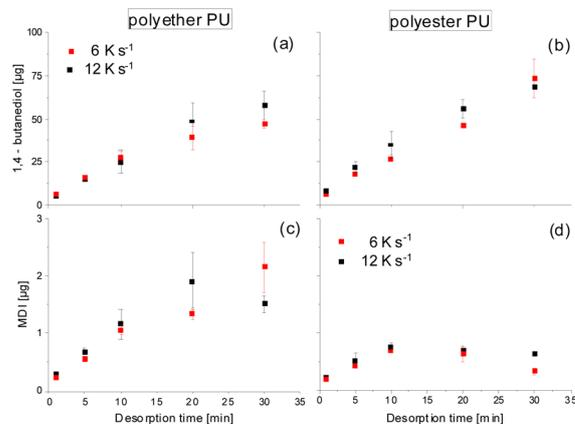
Fig. 3 Time-dependent thermal desorption at  $250\text{ }^\circ\text{C}$  of 1,4-butanediol and MDI from polyether PU (a and c) and polyester PU (b and d) at heating rates of  $6\text{ K s}^{-1}$  (red) and  $12\text{ K s}^{-1}$  (black).
