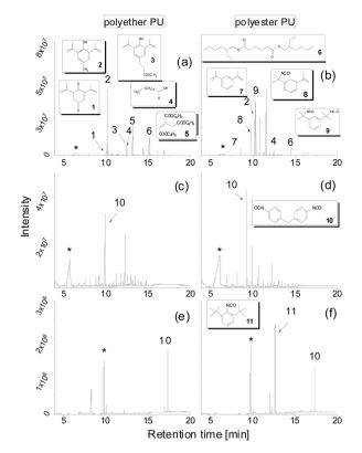
Fig. 1 TD-GC-MS chromatograms of the original polyether and polyester PUs with determined structures (a and b); after purification by precipitation in MeOH using a DB-1 column and thermal desorption for 1 min at 250 °C and 12 K min $^{-1}$  (c and d), and using a polar DB-17ms column and thermal desorption for 10 min at 250  $^{\circ}$ C and 12 K min<sup>-1</sup> (e and f) (the peak of 1,4-butanediol is indicated by an asterisk).
