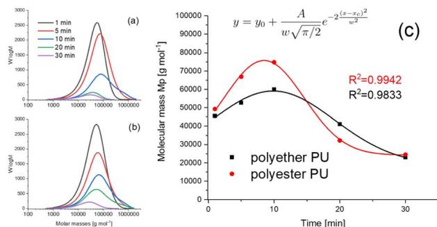
Fig. 5 Molar mass distribution curves of a polyester PU (a) and a polyether PU (b) and the course of the molar mass changes monitored by SEC over time (c) with  $y_0 = 18\,950$  (24 220),  $x_c = 10$  (8),  $w = 19$  (12) and  $A = 9.43 \times 10^6$  ( $7.86 \times 10^6$ ) for the polyether (polyester) PU.
