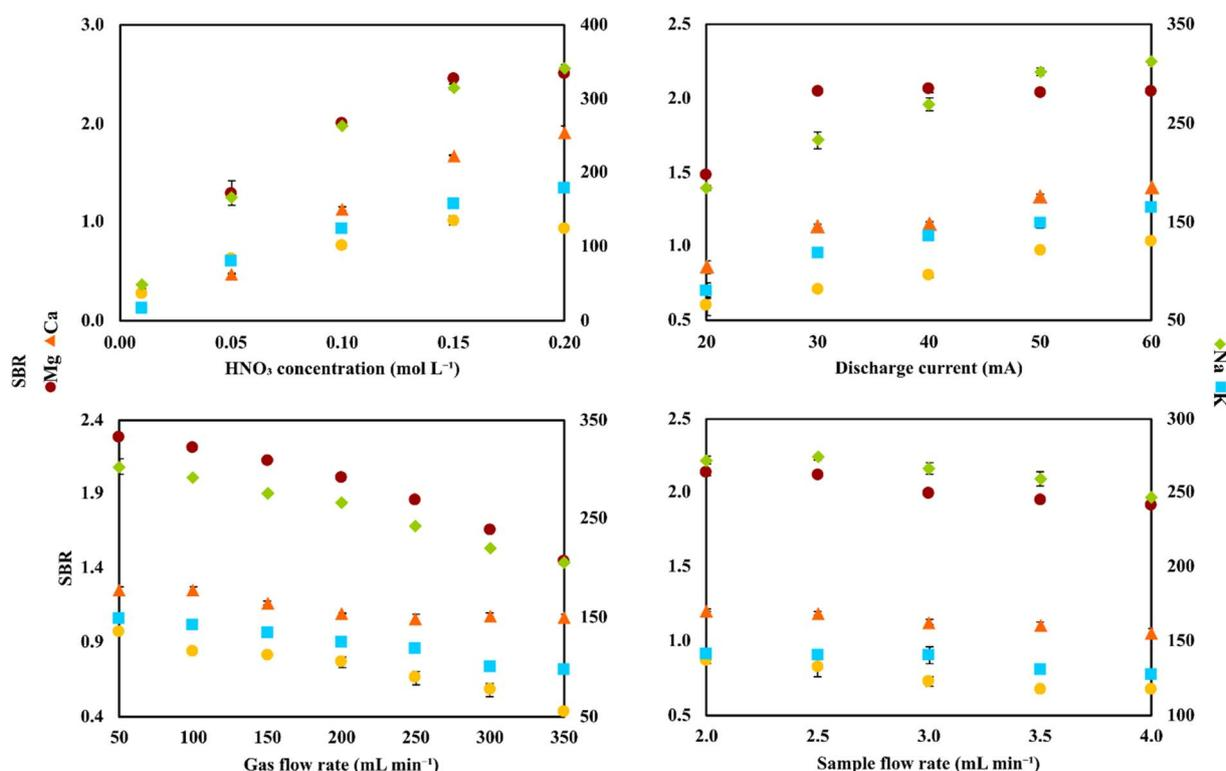
Fig. 2 The impact of HNO<sub>3</sub> concentration, discharge current, gas flow rate, and sample flow rate on the SBR values of the analytical lines of the studied elements for a solution containing only the analytes.
