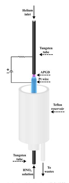
Fig. 1 Schematic drawing of the developed FLC-APGD system.
