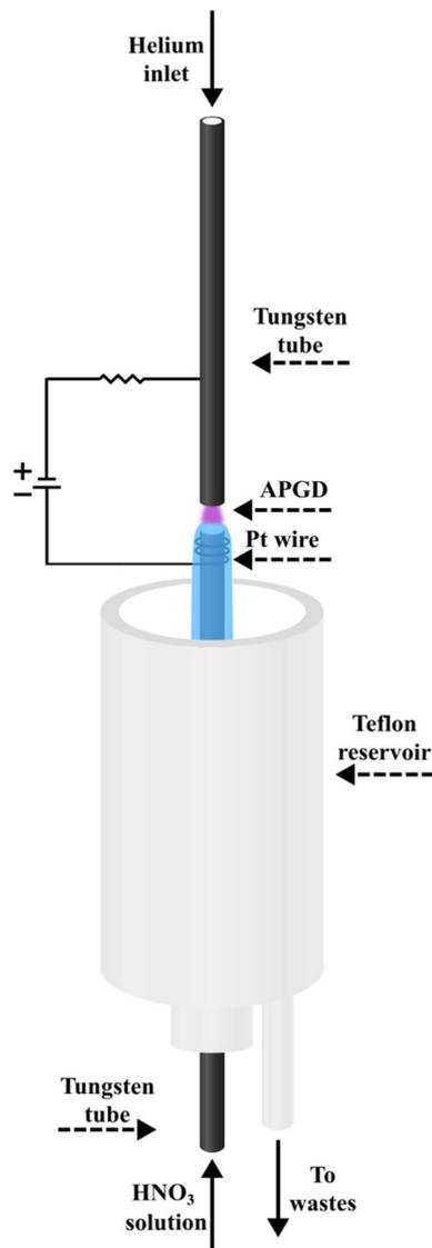
Fig. 1 Schematic drawing of the developed FLC-APGD system.
