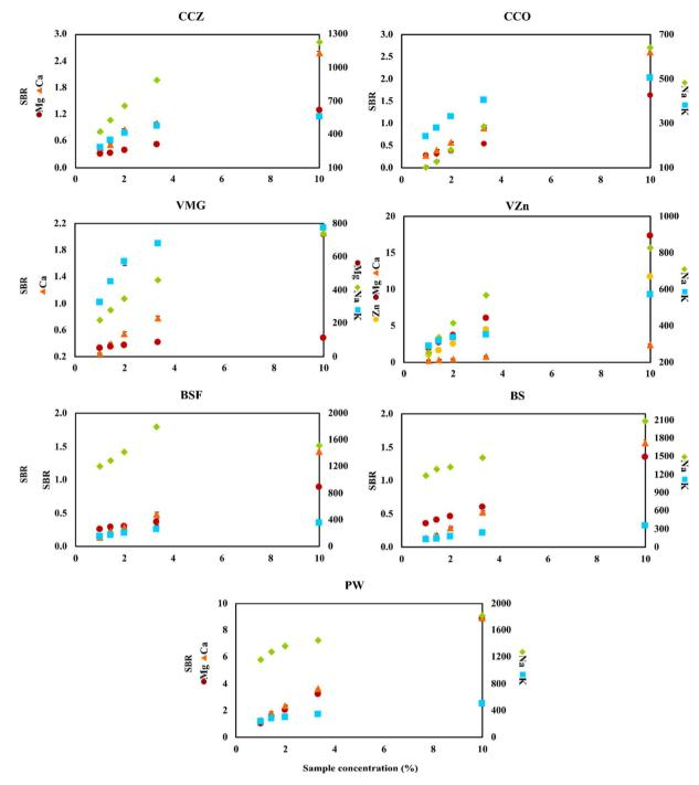
Fig. 3 Impact of the sample dilutions (expressed as percent sample concentration) on the SBR values of the analytical lines of the studied elements for the samples of CCZ, CCO, VMg, VZn, BSF, BS, and PW.
