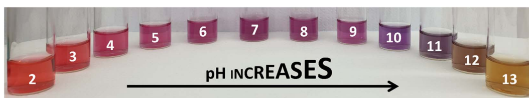
Fig. 3 Colour changes of the BCE in solutions with increasing pH.
