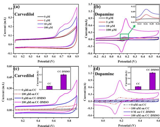
Fig. 3 The CV of CC-DMSO in 0.1 M PBS solution containing (a) different concentrations of CAR and (b) different concentrations of DA. The CV of bare CC and CC-DMSO towards (c) CAR (d) DA. Insets of (c) and (d) show the comparison of sensor response between CC and CC-DMSO at 100  $\mu$ M CAR and DA respectively. The error bar shows the standard deviation of three independent measurements.
