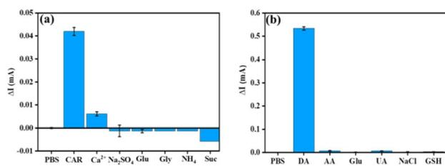
Fig. 5 The selectivity plot showing the CC-DMSO sensor response towards (a) CAR detection in the presence of different interfering molecules such as Glu, Suc, Gly,  $\text{Na}_2\text{SO}_4$ ,  $\text{CaCl}_2$ , and  $(\text{NH}_4)_2\text{SO}_4$ . (b) The selectivity plot towards the DA detection in the presence of different interfering molecules such as AA, Glu, GSH, NaCl and UA. The error bar shows the standard deviation of three independent measurements.
