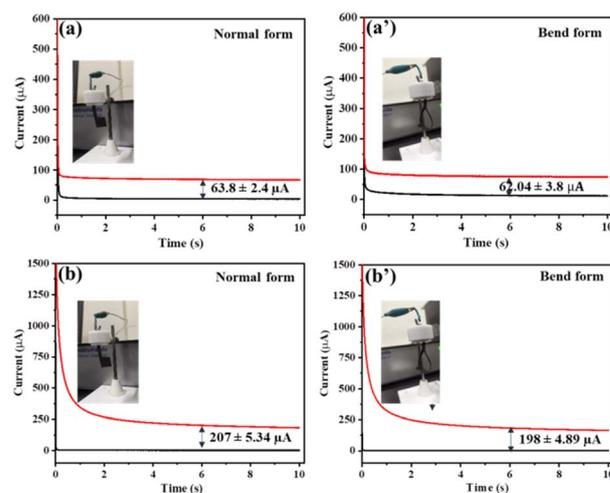
Fig. 6 The chronoamperometric response of the electrode for 10  $\mu\text{M}$  CAR (a and a') and for 10  $\mu\text{M}$  DA (b and b') in the normal and bent forms showing the flexibility of the developed sensor platform.
