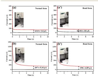
Fig. 6 The chronoamperometric response of the electrode for 10  $\mu$ M CAR (a and a') and for 10 µM DA (b and b') in the normal and bent forms showing the flexibility of the developed sensor platform.
