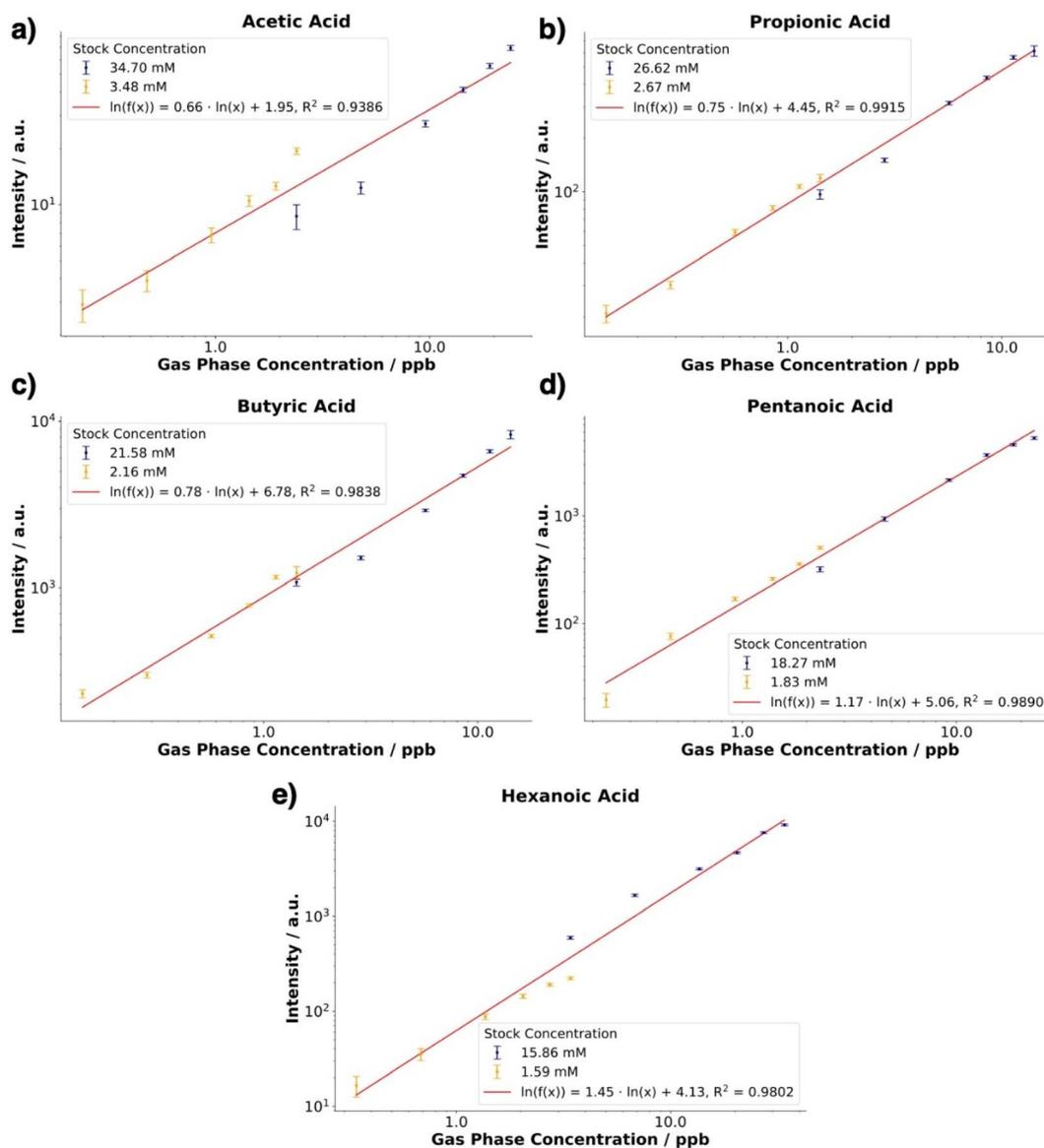
**Fig. 4** Calibration curves obtained for (a) acetic acid, (b) propionic acid, (c) butyric acid, (d) pentanoic acid and (e) hexanoic acid in the gas phase at 95% RH. Each point of the calibration curves corresponds to the average concentration at a specific flow of the four technical replicate measurements (four different flow programs passing through the evaporation chambers). The error bars correspond to the standard error per data point.
