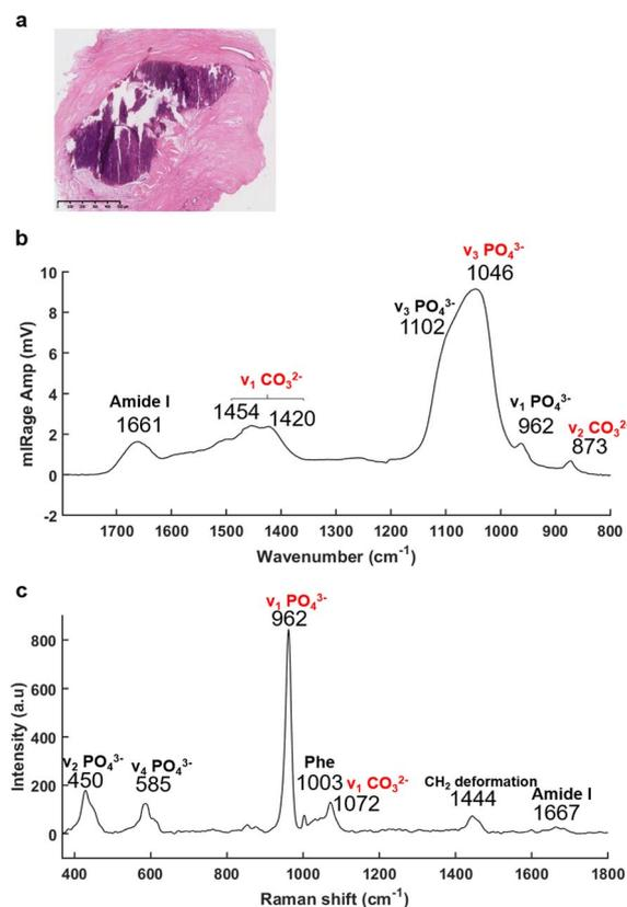
Fig. 3 O-PTIR and Raman spectra acquired in a middle of the microcalcification, at the same time and same spot. (a) White light image of the H&E stained breast tissue section ( $\times 5$  objective), scale bar:  $500\text{ }\mu\text{m}$ . (b) O-PTIR and (c) Raman spectra collected within the BMC (purple staining) between  $1796\text{--}786\text{ cm}^{-1}$  and  $197\text{--}1796\text{ cm}^{-1}$ , respectively.
