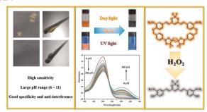
A highly effective "naked eye" colorimetric and fluorimetric curcumin-based fluorescent sensor for specific and sensitive detection of  $H_2O_2$  in vivo and in vitro
