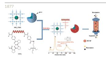
Hybridization of helical poly(phenylacetylene)s bearing L-proline tripeptide pendants into porous silica microspheres as a solvent-tolerable chiral stationary phase for liquid chromatography
