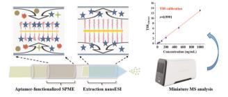
Online hyphenation of in-capillary aptamerfunctionalized solid-phase microextraction and extraction nanoelectrospray ionization for miniature mass spectrometry analysis
