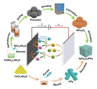
**Fig. 2** Schematic illustration of the preparation process of the NiFe<sub>2</sub>O<sub>4</sub>/PPy nanocomposite. Per Reprinted from Y. Wang, Z. Nie, X. Li, R. Wang, Y. Zhao, and H. Wang, PPy-functionalized NiFe<sub>2</sub>O<sub>4</sub> nanocomposites toward highly selective Pb<sup>2+</sup> electrochemical sensing, *ACS Sustainable Chem. Eng.*, **10**(18), 6082–6093, Copyright (2022) American Chemical Society.
