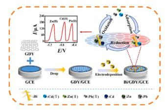
Fig. 4 The preparation of the Bi/GDY/GCE and the application for simultaneous detection of three heavy metal ions<sup>246</sup> (this figure was published in Y. Ai, L. Yan, S. Zhang, X. Ye, Y. Xuan, S. He, X. Wang, W. Sun, Ultra-sensitive simultaneous electrochemical detection of Zn(II), Cd(II) and Pb(II) based on the bismuth and graphdiyne film modified electrode, *Microchem. J.*, **184**, 108186, Copyright Elsevier (2023)).
