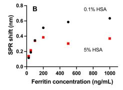
Fig. 6 Calibration curves for different BSA (A) and HSA (B) concentrations in running buffers.
