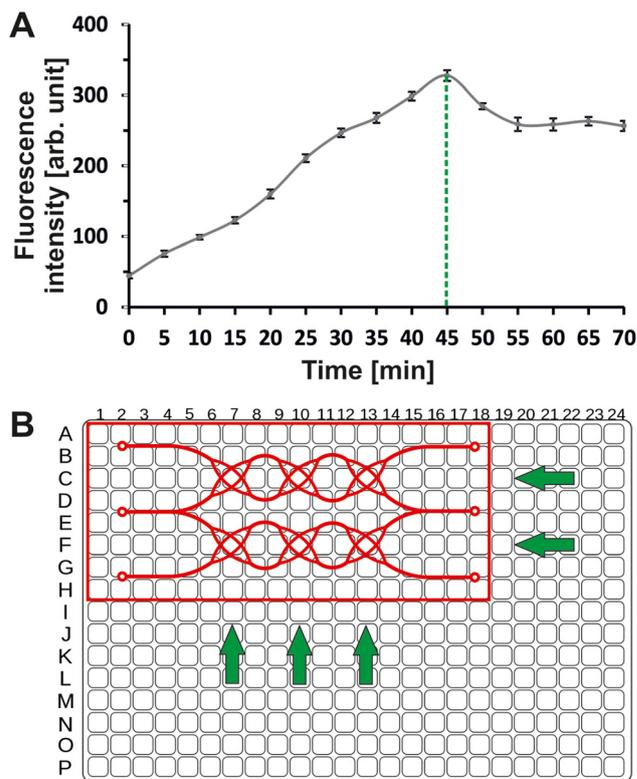
**Fig. 4** (A) Optimization of cell incubation time in the microfluidic system with AlamarBlue reagent. The maximum fluorescence intensity of resorufin was noted after 45 min. (B) Matching the layout of the chambers in the microfluidic system to the arrangement of the wells on a standard 384-well plate.
