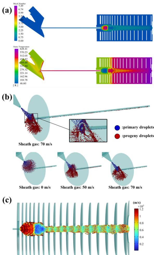
**Fig. 2** (a) Upper: the velocity field (Mach). Lower: the temperature field (K). (b) The trajectories of the primary and progeny droplets in spray area and capillary at different sheath gas. (c) The ion trajectory in the vacuum chamber.
