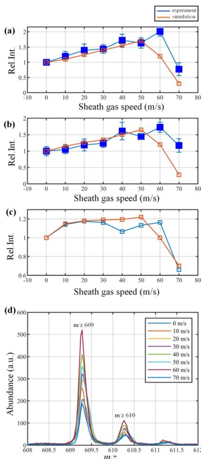
**Fig. 3** (a) Relative intensity of the protonated reserpine (*m/z* 609) and (b) the chemical noise at the sheath gas speed (0–70 m s<sup>-1</sup>). (c) The relative SNR of reserpine. (d) The mass spectra of reserpine at different sheath gas speeds.
