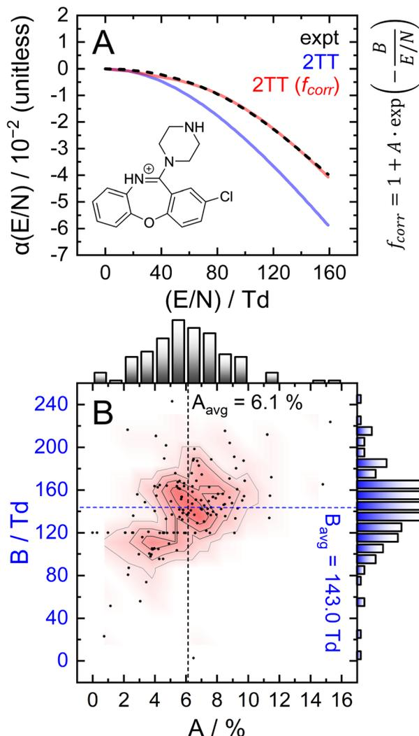
**Fig. 6** Investigation of the empirical correction to 2TT. (A) Comparison of experimental and calculated alpha functions for protonated amoxapine. Optimized parameters are  $A = 4.4\%$  and  $B = 132$  Td. (B) 2D distribution of optimized  $A$  and  $B$  parameters of the empirical correction,  $f_{\text{corr}}$ , over 132 test cases.
