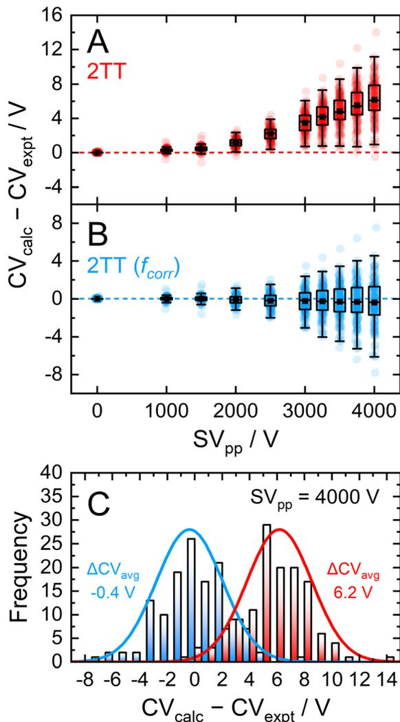
**Fig. 7** Comparison of measured vs. calculated dispersion plots over a range of separation field amplitudes as box plots for (A) uncorrected 2TT and (B) 2TT including the empirical correction employing  $A_{\text{avg}}$  and  $B_{\text{avg}}$ . Panel (C) shows the distribution of CV deviations using the uncorrected and empirically correct 2TT at the highest  $SV_{\text{pp}}$  (4000 V).
