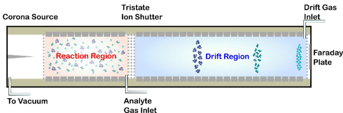
**Fig. 1** A simple diagram of the HiKE-IMS used in this work is shown here. The HiKE-IMS is a variant of a drift tube IMS that is capable of obtaining high reduced electric field strengths independently in the reaction region and drift region, while the ions are detected under drift conditions at a Faraday plate. Therefore, HiKE-IMS is capable of directly measuring first-principles mobilities of ions up to 120 Td.
