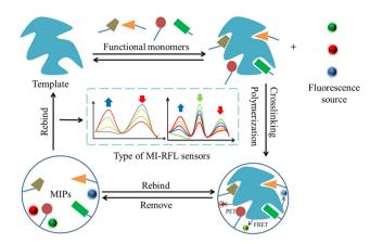
Fig. 1 Schematic illustration of the basic construction and detection process of the MI-RFL sensor.
