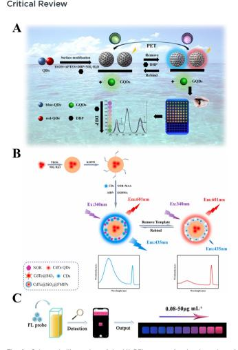
**Fig. 4** Schematic illustration of the MI-RFL sensors for the detection of new pollutants. (A) Sensor construction and detection process for DBP. <sup>98</sup> (B) Preparative strategy of CdTe@SiO<sub>2</sub>@FMIPs for the detection of NOR. <sup>97</sup> (C) The developed smartphone-integrated sensing platform to detect OTC. <sup>80</sup>
