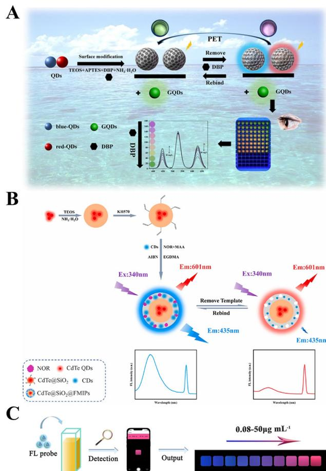
**Fig. 4** Schematic illustration of the MI-RFL sensors for the detection of new pollutants. (A) Sensor construction and detection process for DBP.<sup>98</sup> (B) Preparative strategy of CdTe@SiO<sub>2</sub>@FMIPs for the detection of NOR.<sup>97</sup> (C) The developed smartphone-integrated sensing platform to detect OTC.<sup>80</sup>
