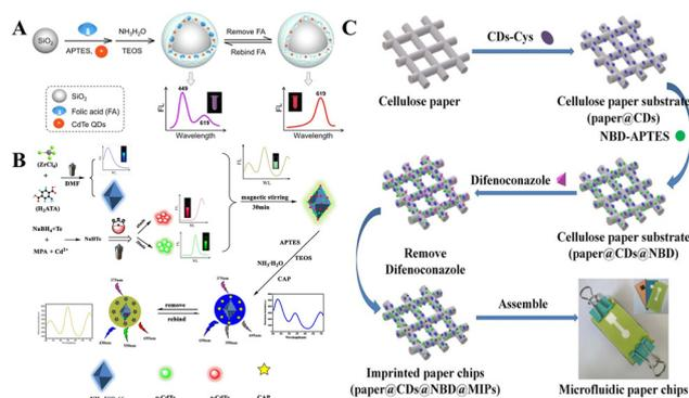
**Fig. 5** Application of MI-RFL sensors in food analysis (A) schematic illustration for the one-pot preparation process of nanoscale core-shell structured FA imprinted ratiometric fluorescence sensor and possible detection principle.<sup>58</sup> (B) Preparation and detection procedure of ternary-emission MOF@g-CdTe@r-CdTe@MIP.<sup>81</sup> (C) Construction of MIP-based ratiometric fluorescent microfluidic paper chip.<sup>117</sup>
