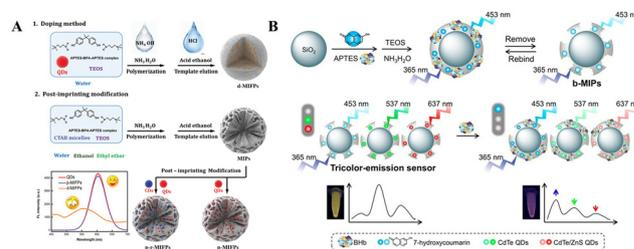
**Fig. 3** Post-imprinting strategies. (A) Process for the preparation of MIPs *via* the doping method and post-imprinting modification method.<sup>76</sup> (B) Schematic illustration for the preparation of blue-emission MIPs (b-MIPs) and the construction of a triple-color emission sensor by mixing blue-, green- and red-emission MIPs (b-, g-, and r-MIPs) at an optimized volume ratio of 50/110/60.<sup>79</sup>
