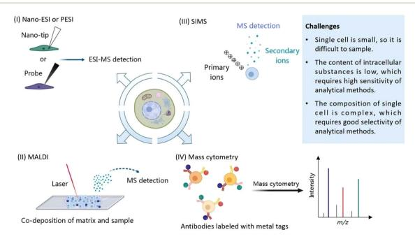
Fig. 1 Challenges of single cell analysis by mass spectrometry: (I) Nano-ESI or PESI, (II) SIMS, (III) MALDI, (IV) Mass cytometry.
