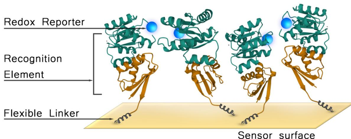
**Fig. 1** Scheme illustrating the three main components of protein-based electrochemical biosensors: the recognition elements engineered within a redox reporter and attached to an electrode surface using a flexible linker.
