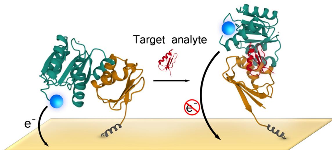
**Fig. 2** Scheme illustrating how binding of the recognition element to the target analyte leads to protein conformational changes and consequently alters the relative position of redox reporter to the electrode surface. This alteration in redox reporter position, in this case moving far away from the electrode surface, results in a measurable voltammetric current which is proportional to target analyte concentration.
