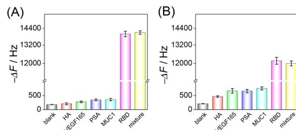
**Fig. 4** Selectivity of the HF-QCM aptasensor (A) and immunosensor (B) for the RBD assay. RBD, 100  $\text{pg mL}^{-1}$ ; interferent, 1  $\text{ng mL}^{-1}$ ; the mixture contained the RBD (100  $\text{pg mL}^{-1}$ ) and four interferences (each interferent, 1  $\text{ng mL}^{-1}$ ).
