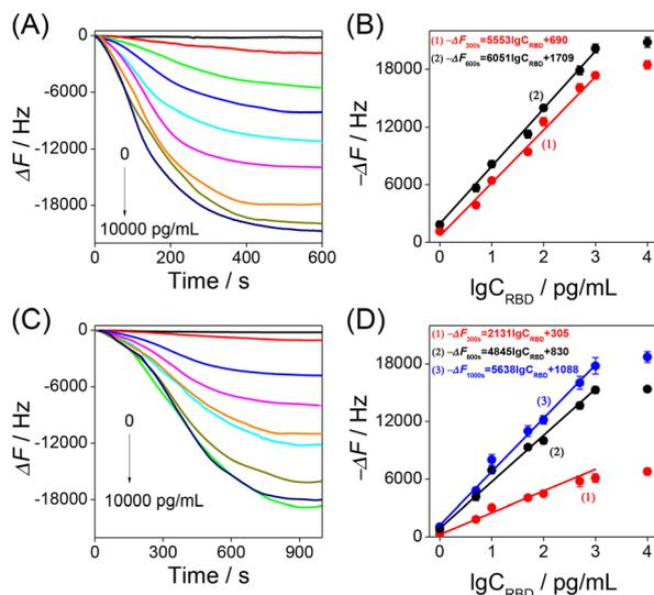
**Fig. 3** Frequency changes of the HF-QCM aptasensor (A) and immunosensor (C) with different concentrations of the RBD: 0, 1, 5, 10, 50, 100, 500, 1000, and 10000  $\text{pg mL}^{-1}$ . Dependence of  $-\Delta F$  values of the HF-QCM aptasensor (B) and immunosensor (D) at definite recognition times on the logarithm of RBD concentrations.
