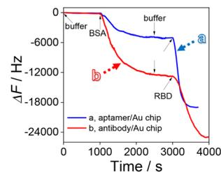
**Fig. 2** Real-time responses of the aptamer (antibody)-modified QCM Au chip for the following processes: washing with buffer, blocking the surface with BSA, washing with buffer, and specific recognition of the RBD.  $C_{\text{RBD}} = 100 \text{ pg mL}^{-1}$ .
