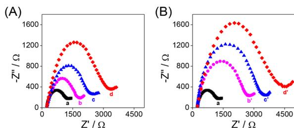
**Fig. 1** Nyquist plots of different modified QCM Au chips in  $5 \text{ mM } [\text{Fe}(\text{CN})_6]^{3-/4-}$  (1 : 1) solution containing  $0.1 \text{ M KCl}$  (frequency,  $10^5\text{--}0.1 \text{ Hz}$ ). (A) (a) Bare Au chip, (b) aptamer/Au chip, (c) BSA/aptamer/Au chip, and (d) RBD/BSA/aptamer/Au chip; (B) (a) bare Au chip, (b') antibody/Au chip, (c') BSA/antibody/Au chip, and (d') RBD/BSA/antibody/Au chip.  $C_{\text{RBD}} = 100 \text{ pg mL}^{-1}$ .
