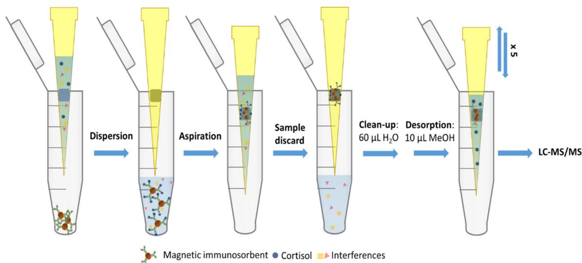
**Fig. 2** Scheme of the proposed analytical method.
