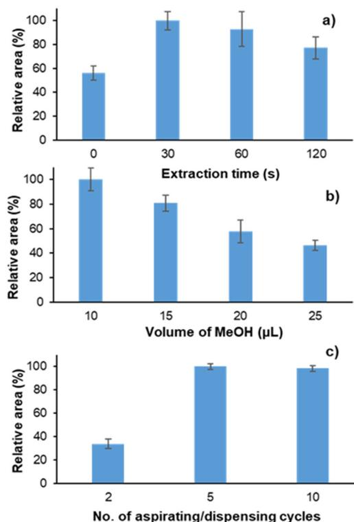
**Fig. 4** Optimization of the extraction and desorption variables: (a) the extraction time; (b) the volume of MeOH; and (c) the number of dispersion aspirating/dispensing cycles. The error bars show the standard deviation ( $N = 3$ ).
