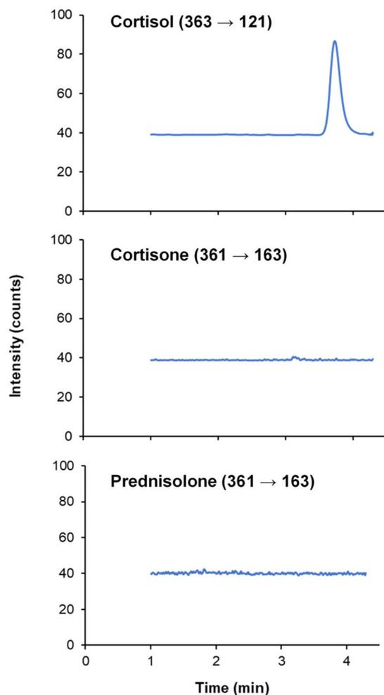
**Fig. 5** Chromatogram of a PBS solution spiked with 10 ng mL<sup>-1</sup> of cortisol, cortisone and prednisolone after the magnetic-based pipette tip microextraction method.
