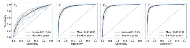
Fig. 3 By-patient ROC curves for model type ConvBMaxP $^2$ -L-MLP trained on dataset A across the representations  $F_R$ , F,  $T_R$ , T (left to right): mean curve (blue) and 10 curves (grey) corresponding to the independent experiments. Mean ROC curve is obtained by averaging sensitivity and specificity for a fixed threshold across 10 models.
