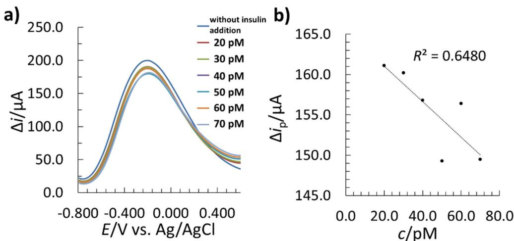
**Fig. 11** The electrochemical performance of the NIP-SPCE in a single drop: (a) the SWV voltammograms of the NIP-SPCE measured in 0.01 M PBS (pH 7.2) containing the 5 mM  $[\text{Fe}(\text{CN})_6]^{3-/4-}$  redox probe with different concentrations of insulin, and (b) the corresponding linear calibration curve of  $\Delta i_p$  as a function of the insulin concentration for the electrochemical response on the NIP-SPCE sensor.
