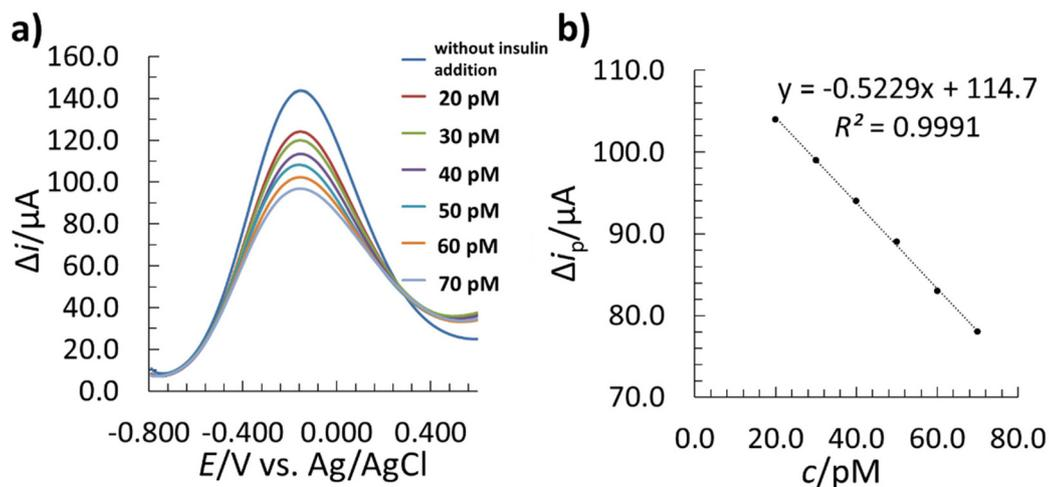
**Fig. 10** The electrochemical performance of the MIP-SPCE for rebinding insulin in a single drop: (a) SWV voltammograms of the MIP-SPCE measured in 0.01 M PBS (pH 7.2) containing the 5 mM  $[\text{Fe}(\text{CN})_6]^{3-/4-}$  redox probe with different concentrations of insulin, (b) the corresponding linear calibration curve ( $\Delta i_p$  stands for the SW peak height).
