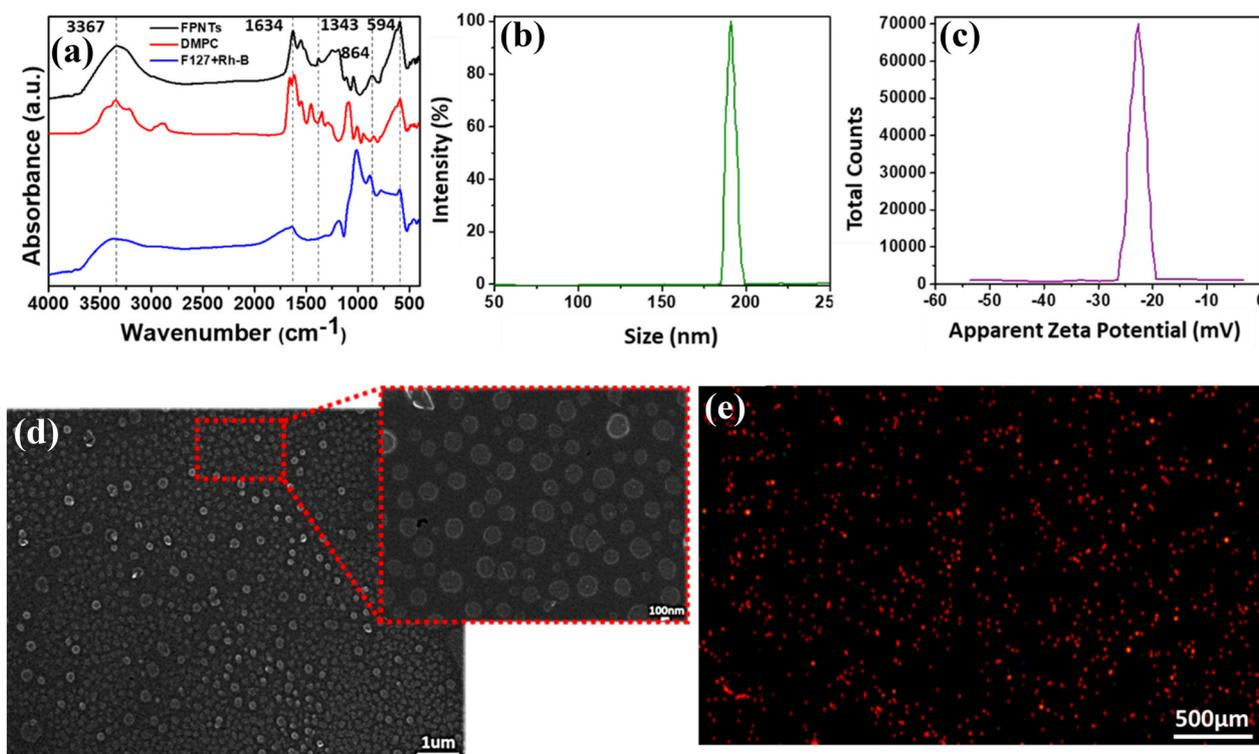
**Fig. 2** Structural and morphological characterization of FPNTs using the (a) FTIR spectra of the FPNTs, dye micelle polymer complex (DMPC), and F-127 + Rh-B dye. (b) Hydrodynamic diameter distribution and (c) zeta potential of FPNTs. (d) SEM image of FPNTs. (e) Fluorescence image of FPNTs.
