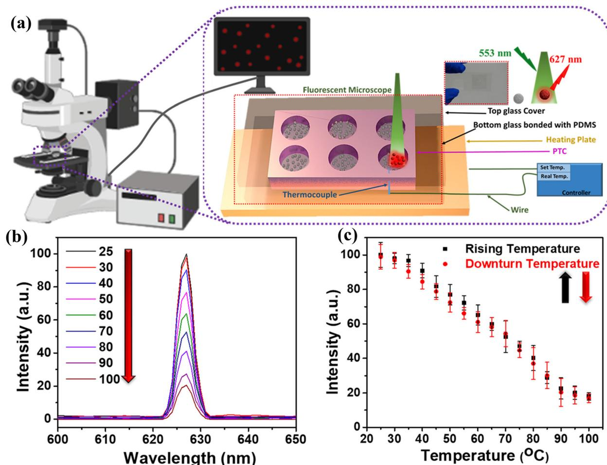
**Fig. 3** Temperature dependence of the fluorescence emission from the Rh-B encapsulated polymeric nanoparticles, FPNTs, dissolved in DI water. (a) Experimental set-up for the calibration of FPNTs. (b) Temperature-related emissions of the temperature-sensitive FPNTs using a fluorospectrometer dispersed in water in the temperature range of 25–100 °C. (c) Average fluorescence lifetime versus temperature during repeated heating and cooling and the corresponding linear regression.
