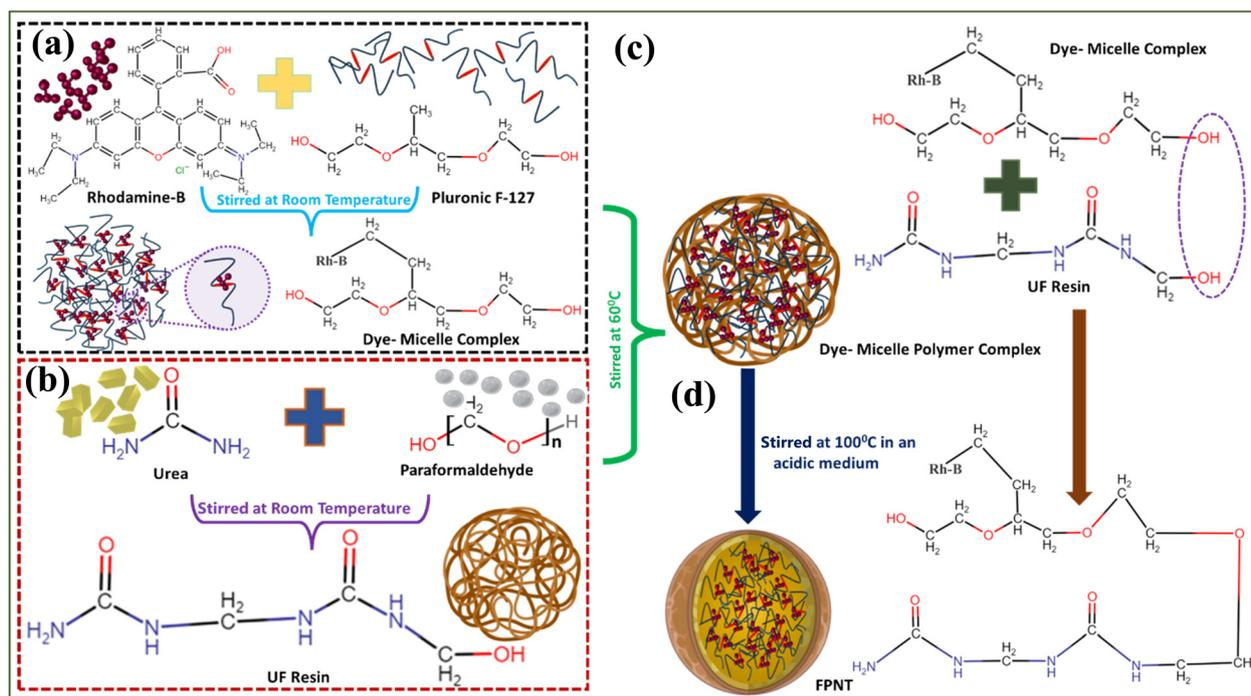
**Fig. 1** Schematic illustration of the preparation of FPNTs. (a) Micelle formation of the Rh-B dye and Pluronic F-127 polymer by a hydrophobic and hydrophobic interaction mechanism. (b) Formation of a urea and paraformaldehyde resin, which acts as a cross-linker. (c) Incorporation of a dye micelle in UPF resin. (d) Condensation of the hydroxyl group results in FPNTs.
