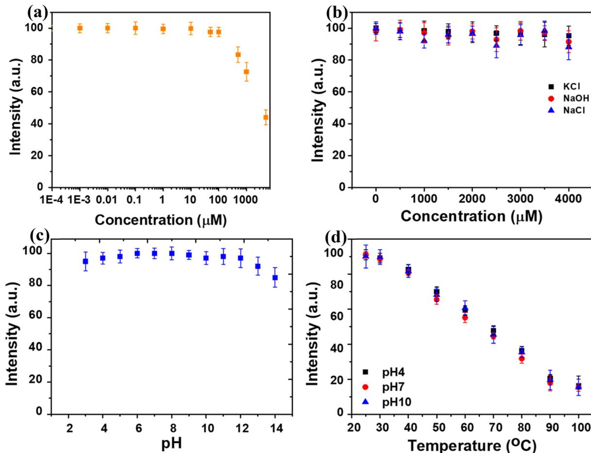
**Fig. 5** The environmental behavior of FPNTs. (a) Fluorescence intensity of FPNTs in  $\text{H}_2\text{O}_2$  solution with different concentrations. (b) Fluorescence intensity of FPNTs in KCl, NaOH, and NaCl solutions with different concentrations at room temperature. (c) Fluorescence intensity of FPNTs at various pH values. (d) Temperature sensing properties of FPNTs in solutions at various pH values.
