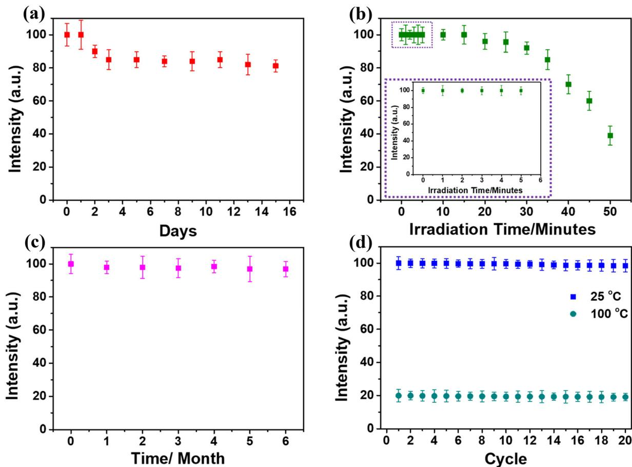
**Fig. 4** Performance assessment of FPNTs. (a) Dye leakage from the fabricated FPNTs. (b) Fluorescence lifetime of FPNTs as a function of irradiation time. (c) Fluorescence intensity of FPNTs vs. time. (d) Lifetime of FPNTs during repeated heating and cooling (cycling the temperature twenty times between 25 and 100 °C).
