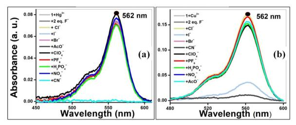
Fig. 5 (a) UV-visible spectra of  $\mathbf{1} + \mathrm{Hg}^{2+}$  ([1] = 10  $\mu$ M,  $\mathbf{1} : \mathrm{Hg}^{2+} = 1 : 1$ ) with different anions in acetonitrile—water (1 : 1) medium. (b) UV-visible spectra of  $\mathbf{1} + \mathrm{Cu}^{2+}$  ([1] = 10  $\mu$ M,  $\mathbf{1} : \mathrm{Cu}^{2+} = 1 : 1$ ) with different anions in acetonitrile—water (1 : 1) medium.
