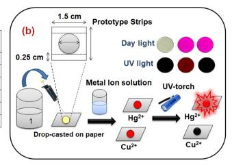
Fig. 7 (a) Detection limit of 1 for  $Cu^{2+}$  and  $Hq^{2+}$  in different natural water sources. (b) Photographs of the test strips made from 1 (50  $\mu$ M) for the detection of Cu<sup>2+</sup> and Hg<sup>2+</sup> both under daylight and under UV lamp (365 nm).
