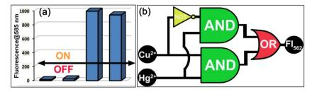
Fig. 11 (a) Optical bar responses and (b) corresponding schematic logic presentation of the TRANSFER logic gate based on the fluorescence responses of 1 at 562 nm, considering Cu<sup>2+</sup> and Hg<sup>2+</sup> as chemical inputs.
