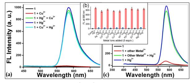
Fig. 3 (a) Response of 1 towards the alternate addition of  $Hq^{2+}$  and  $Cu^{2+}$  ion (b) in the individual presence of other cations (in excess) monitored at 585 nm. (c) Versatile selectivity plot of 1 towards Hg<sup>2+</sup> in an ionic mixture.
