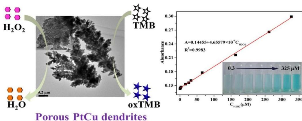
Fig. 3 Schematic diagram of HPtCuDs catalysis of the classical peroxidase substrate TMB by  $\text{H}_2\text{O}_2$  and linear calibration plot for  $\text{H}_2\text{O}_2$  detection.<sup>84</sup>
