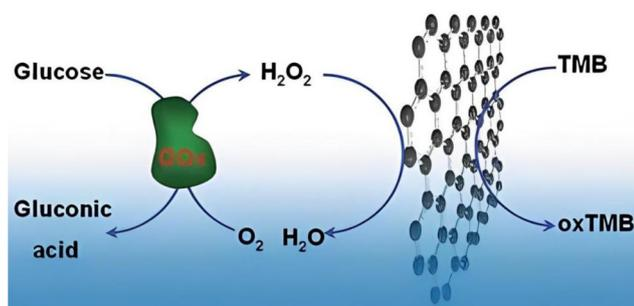
Fig. 11 Schematic diagram of a colorimetric approach for the detection of glucose based on GOx and the GO-COOH catalyzed TMB- $\text{H}_2\text{O}_2$  system.<sup>122</sup>
