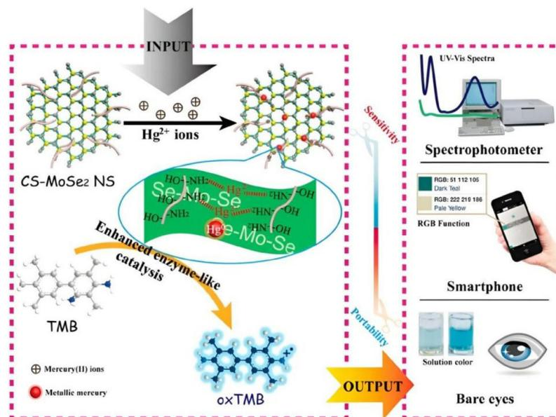
Fig. 10 Versatile colorimetric detection diagram of  $\text{Hg}^{2+}$  based on CS-MoSe<sub>2</sub> nanosheets.<sup>119</sup>
