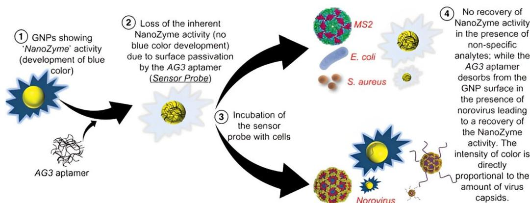
Fig. 1 Schematic diagram of the nanozyme aptasensor prepared by adapting Au NPs to norovirus aptamer.<sup>62</sup>
