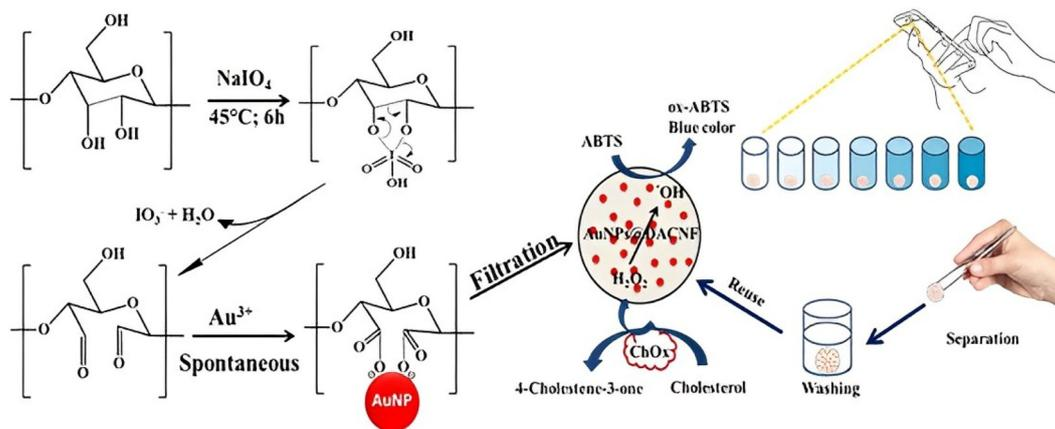
Fig. 2 Schematic illustration of the preparation of paper-based Au NPs@DACNF sensor and the colorimetric detection of cholesterol assisted by smartphone.<sup>67</sup>
