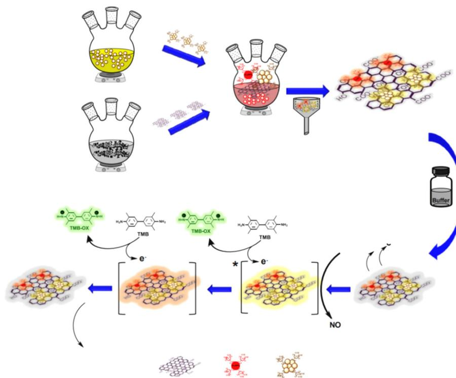
Fig. 12 Schematic illustration of the synthesis of Au NP-CeO<sub>2</sub> NP@GO nanozymes and their use for colorimetric detection of nitrite.<sup>126</sup>
