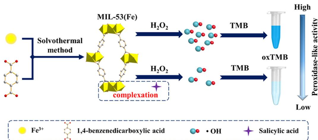
Fig. 18 Schematic diagram of MIL-53(Fe) synthesized using the solvothermal method and the colorimetric detection of SA based on MIL-53(Fe) MOFs nanozymes.<sup>148</sup>
