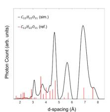
**Fig. 4** Reconstruction of simulated diffractogram of the  $C_{12}H_{22}O_{11}$  sample investigated in Fig. 3. Sample location is 225–235 mm from the X-ray source with approximate corresponding diffraction angle,  $2\theta$  = 5.8°.
