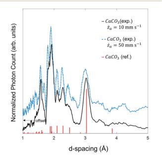
Fig. 10 Reconstruction of experiment diffractogram of the CaCO<sub>3</sub> sample investigated in Fig. 9. Predicted sample location ~ 302 mm with approximate corresponding diffraction angle,  $2\theta = 6.6^{\circ}$ .
