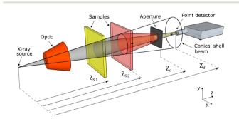
Fig. 1 Concept image of the swept aperture system with crystalline samples at z-axis positions,  $z_{s,1}$  and  $z_{s,2}$ ; circular aperture at  $z_a$  and energy-resolving detector at  $z_d$ . The aperture selects upper limits in z-space observed by the detector.
