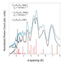
**Fig. 8** Reconstruction of experiment diffractogram of the  $C_{12}H_{22}O_{11}$  sample investigated in Fig. 7, with aperture velocities of 10 mm s<sup>-1</sup> (black, solid) and 50 mm s<sup>-1</sup> (blue, dashed). Predicted sample location is  $\sim$ 229 mm from the X-ray source.
