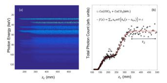
Fig. 5 Monte Carlo simulation of multiple samples:  $Ca(OH)_2$  at 160-175 mm and  $CaCO_3$  at 280-295 mm with (a) energy-resolved detector intensity at each maximum observed *z*-axis position and (b) energy-integrated detector intensity with a sum of error functions model fitted and integration periods,  $\tau_1$  and  $\tau_2$ .
