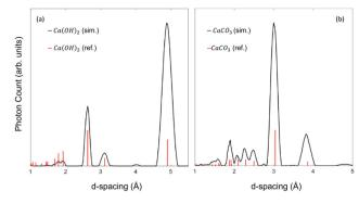
Fig. 6 Reconstruction of simulated diffractograms of the (a) Ca(OH)<sub>2</sub> and (b) CaCO<sub>3</sub> samples investigated in Fig. 5. Sample locations are (a) ~161 mm from the X-ray source with approximate corresponding diffraction angle,  $2\theta = 5.1^{\circ}$  and (b) ~282 mm from the X-ray source with approximate corresponding diffraction angle,  $2\theta = 6.6^{\circ}$ .
