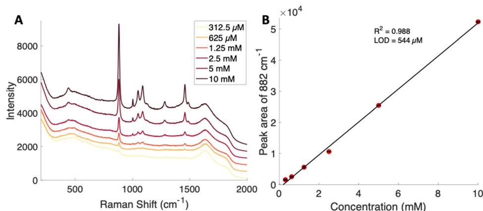
**Fig. 3** (A) Average spontaneous spectra from various concentrations of glucose–PBA. The spectra are offset for clarity. (B) Raman based calibration curve for glucose–PBA using the area of the 882 cm<sup>-1</sup> peak showing a limit of detection of 544 μM. Error bars included are the standard deviation from replicate measurements.
