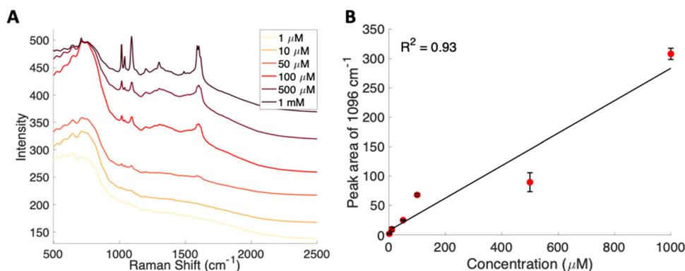
**Fig. 4** (A) Average spectra from various concentrations of glucose–PBA flowing over a substrate. The spectra are offset for clarity. (B) SERS based calibration curve for glucose–PBA using the area of the 1096 cm<sup>-1</sup> peak. Error bars included are the standard deviation from replicate measurements.
