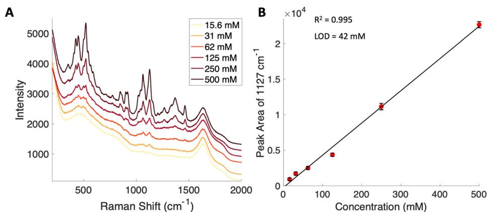
**Fig. 1** (A) Average spontaneous spectra from the various concentrations of glucose noted in the legend. The spectra are offset for clarity. (B) Raman based calibration curve for glucose determined using the area of the  $1127\text{ cm}^{-1}$  peak indicates a limit of detection of 42 mM. Error bars included are the standard deviation from replicate measurements ( $n = 3$ ).
