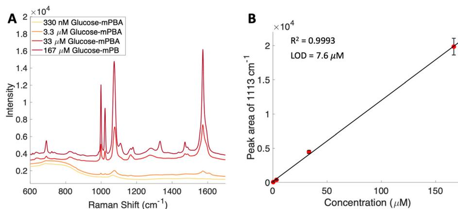
Fig. 7 (A) Average spectra from substrates functionalized with various concentrations of glucose-mPBA conjugate. The spectra are offset for clarity. (B) SERS based calibration curve for glucose-mPBA using the area of the 1113 cm<sup>-1</sup> peak showing a limit of detection of 7.6 μM. Error bars included are the standard deviation from replicate measurements.
