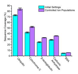
Fig. 4 Sequence coverage for proteins at initial settings and updated settings with controlled ion populations. Ion populations were reduced *via* decreased accumulation time for all proteins. In addition to these altered accumulation times, the sample concentration for BSA and carbonic anhydrase were also decreased.
