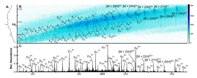
Fig. 3 (A) CIDtims mass spectrum of  $0.5 \mu M$  carbonic anhydrase (B) mobility spectrum of carbonic anhydrase following CIDtims (C) 2D-IMS-MS plot of dissociated carbonic anhydrase with accumulation time of 20 ms and tunnel-in pressure of 1.5 mbar.
