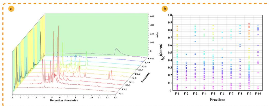
Fig. 2 Orthogonality evaluation of the established 2D chromatography system. (a) Separation effect of *T. wilfordii* extract in 2D RP  $\times$  SFC system; (b) 2D separation orthogonality plan of RP  $\times$  SFC.
