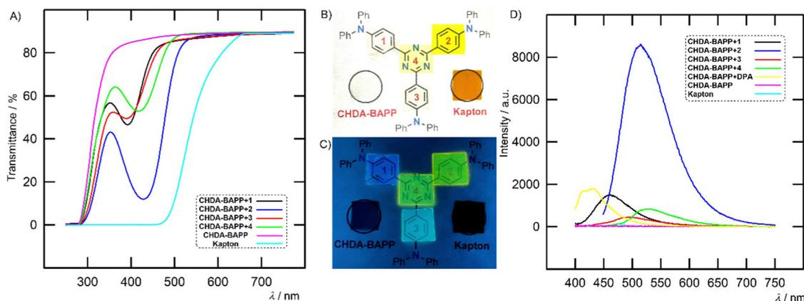
Fig. 9 Transmittance of PI films (A), colour of CHDA-BAPP and films doped with 1–4 (numbered in red) under daylight (B) and 254 nm irradiation (C) and emission spectra of films (D). The spectra and native films (CHDA-BAPP doped with 0.1% of 1–4) are shown along with the reference Kapton film.
