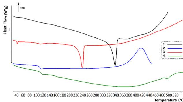
Fig. 2 DSC curves of compounds **1–4** obtained using a heating rate of 10 °C min<sup>-1</sup> under N<sub>2</sub>.
