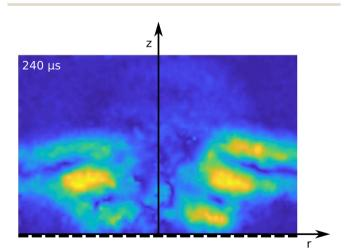
Fig. 8 Shear measured in the left and right quadrant generated here by a cavitation bubble with  $\gamma = 0.48$ . The solid boundary is shown with a dashed line below the frame.
