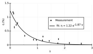
Fig. 7 Efficiency of the shear generation as a function of stand-off distance. Fitting an exponential curve as  $\eta = a \exp(b\gamma)$ , we show shear efficiency reduces exponentially with  $\gamma$  as  $\eta = a \exp(b\gamma)$  with a = 1.22 and b = -1.87 (RMSE = 0.1241).
