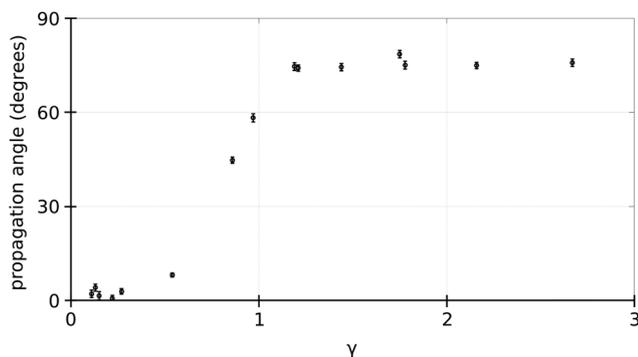
Fig. 6 Angle of shear wave Poynting vector with respect to the axis of symmetry. For  $\gamma < 0.5$ , the shear wave propagates almost parallel to the axis of symmetry. For  $\gamma > 1$  it propagates at an angle of about  $75^\circ$  with respect to the axis of symmetry. In the transition regime ( $0.5 \leq \gamma \leq 1$ ) both shear waves are generated with similar amplitude.
