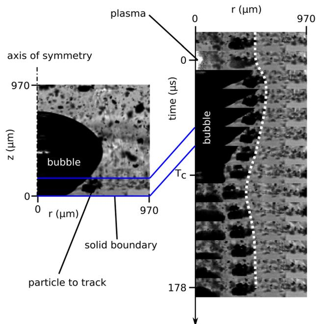
Fig. 5 Study of origin of shear wave generation for the small stand-off case  $\gamma = 0.15$ . The temporal development of a selected region indicated with a blue box is shown, and a selected particle is tracked in time with the dashed line. The sudden changes in the slope of the dashed line at early expansion and late collapse stage indicate shear generation.
