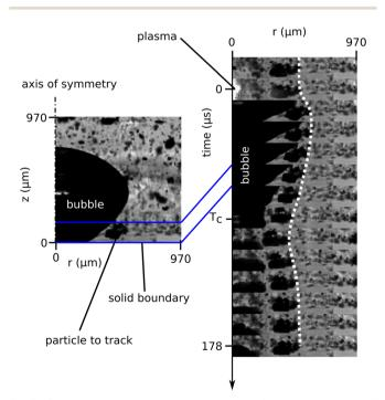
Fig. 5 Study of origin of shear wave generation for the small stand-off case  $\gamma$  = 0.15. The temporal development of a selected region indicated with a blue box is shown, and a selected particle is tracked in time with the dashed line. The sudden changes in the slope of the dashed line at early expansion and late collapse stage indicate shear generation.
