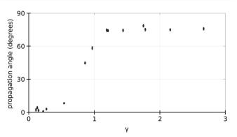
Fig. 6 Angle of shear wave Poynting vector with respect to the axis of symmetry. For  $\gamma$  < 0.5, the shear wave propagates almost parallel to the axis of symmetry. For  $\gamma\,>\,1$  it propagates at an angle of about  $75^\circ$  with respect to the axis of symmetry. In the transition regime (0.5  $\leq \gamma \leq$  1) both shear waves are generated with similar amplitude.
