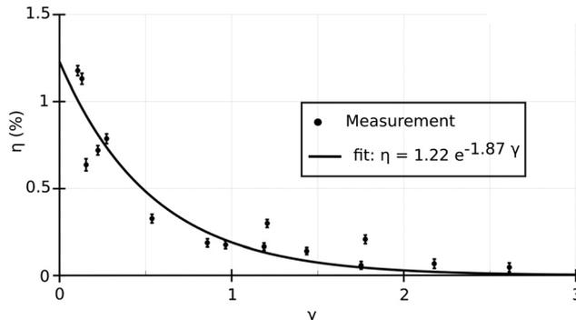
Fig. 7 Efficiency of the shear generation as a function of stand-off distance. Fitting an exponential curve as  $\eta = a \exp(b\gamma)$ , we show shear efficiency reduces exponentially with  $\gamma$  as  $\eta = a \exp(b\gamma)$  with  $a = 1.22$  and  $b = -1.87$  (RMSE = 0.1241).
