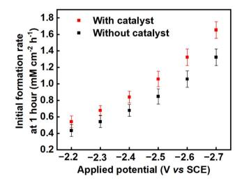
Fig. 6 The formation rates of oxalic acid on a Pb cathode in propylene carbonate over the first hour of electrolysis across the range of applied voltages from -2.2 V to -2.7 V vs. SCE in; an uncatalysed system (black squares) and a system catalysed using benzonitrile (red squares).
