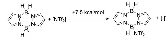
Scheme 7 Free energy change for iodide/ $[\text{NTf}_2]^-$  exchange.
