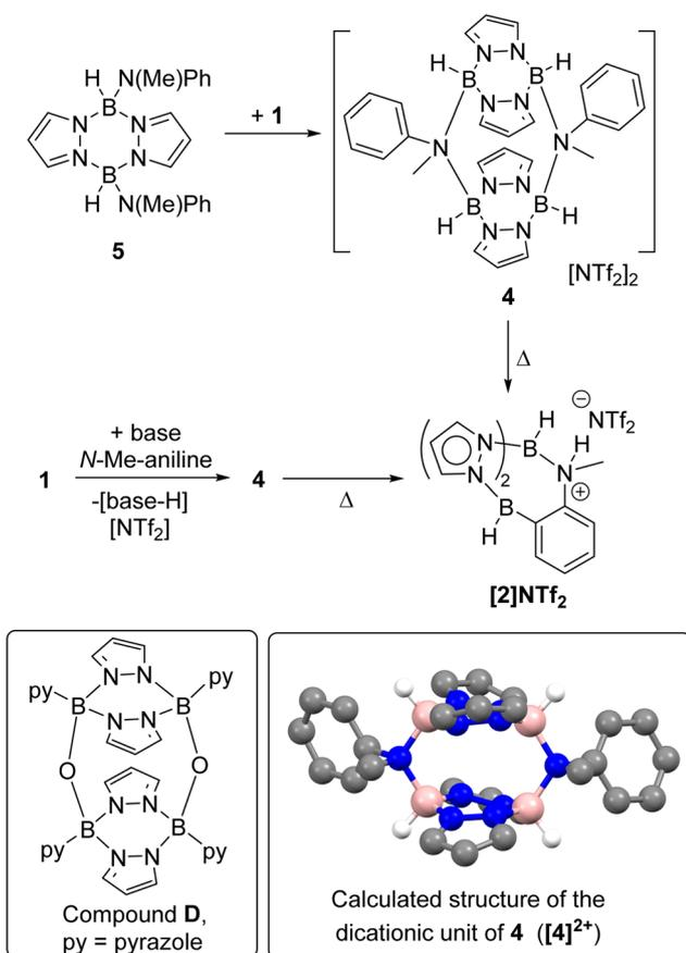
Scheme 3 Top, the formation of **4**, from combination of **1** and **5**; middle, the formation of **4** during BDB and its subsequent conversion into [2]NTf<sub>2</sub>. Inset bottom left, the previously reported oxo bridged dimeric pyrazabole, **D**; inset bottom right the calculated structure of [4]<sup>2+</sup> showing only the hydrogens bonded to boron for clarity, pink = boron, blue = nitrogen, grey = carbon, white = hydrogen.
