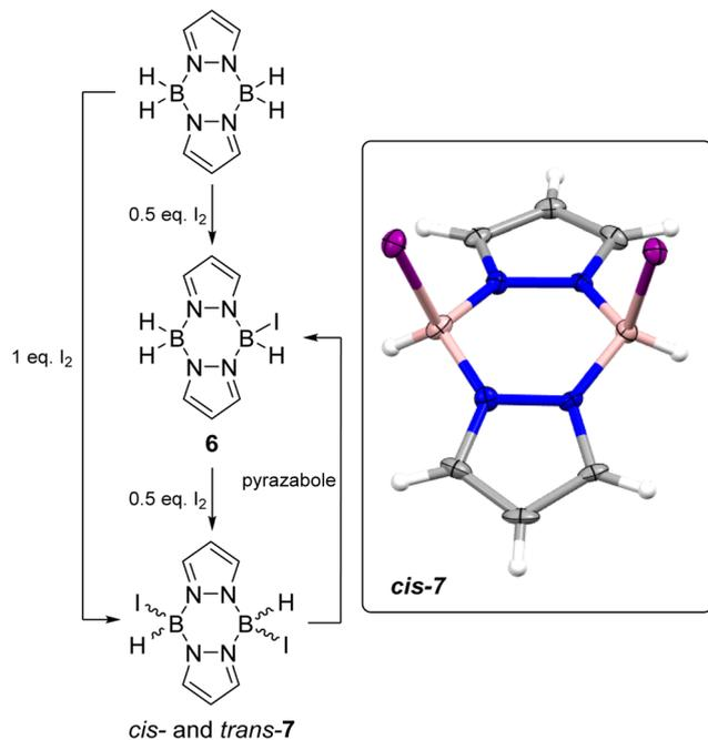
**Scheme 4** Left, formation of mono- (**6**) and diiodo-pyrazabole (**7**). Inset right, the solid state structure of *cis*-**7**, ellipsoids at 50% probability. Blue = nitrogen, pink = boron, purple = iodine, grey = carbon, white = hydrogen.
