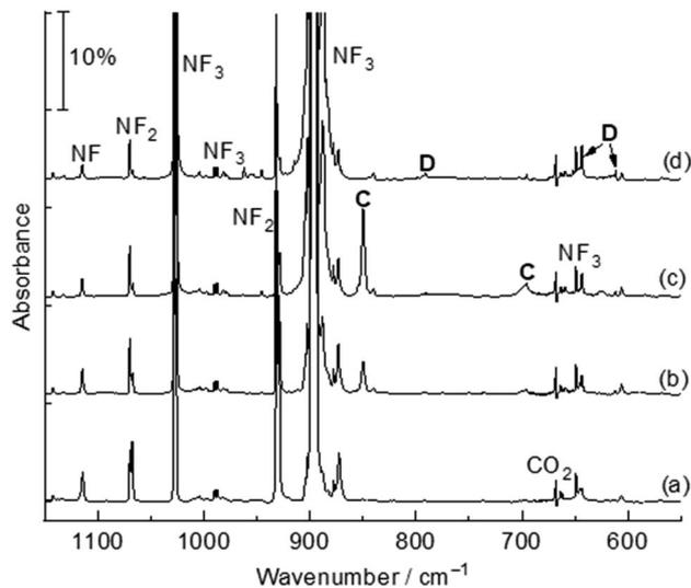
Fig. 2 Infrared spectra in the 1150–550  $\text{cm}^{-1}$  region from co-deposition of laser-ablated Pt atoms with 0.5%  $\text{NF}_3$  in argon. (a) After 60 min of sample deposition, (b) after annealing to 15 K, (c) after annealing to 20 K, and (d) after 10 min of blue LED ( $\lambda = 470$  nm) light irradiation. C:  $\text{Pt}(\text{NF}_3)$ ; D:  $\text{FNPtF}_2$ .
