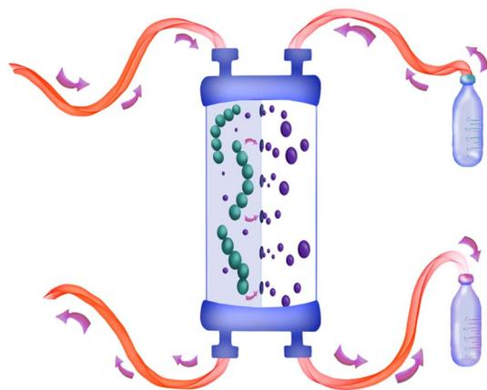
Fig. 1 The general principle of the inline dialysis module used in this work. A polymer is synthesised and brought in continuously *via* the inlet. The unreacted monomer is removed *via* membrane dialysis.
