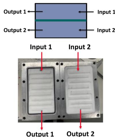
Fig. 2 Design of the continuous flow dialysis block used in this work.
