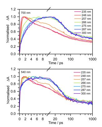
Fig. 3 Kinetic traces of the transient absorption spectra of 20 mM aqueous phenolate at a probe wavelength of 700 nm (top) and 540 nm (bottom) and displayed pump wavelengths. Data have been normalised to maximum  $\Delta A$ .
