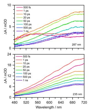
Fig. 2  $\,$  480–720 nm transient absorption spectra of 20 mM aqueous phenolate at displayed pump-probe delays following photoexcitation at 287 nm (top) and 235 nm (bottom). The broad absorption centered around 700 nm is attributed to solvated electrons and the absorption feature with a peak around 540 nm is attributed to the S $_1$  state of phenolate.  $^{12}$
