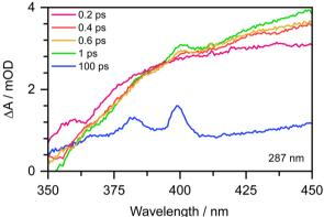
Fig. 7 350–450 nm transient absorption spectra of 20 mM aqueous phenolate at displayed pump-probe delays following photoexcitation at 235 nm (top) and 287 nm (bottom). The dashed vertical highlights the peak at 427 nm described in the main text.
