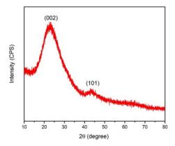
Fig. 3 P-XRD spectrum of AC-SO<sub>3</sub>H.
