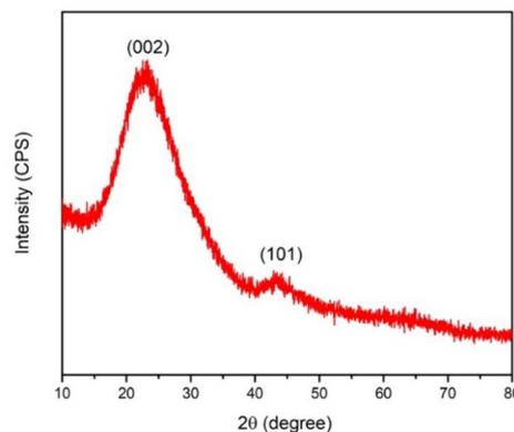
Fig. 3 P-XRD spectrum of AC-SO<sub>3</sub>H.
